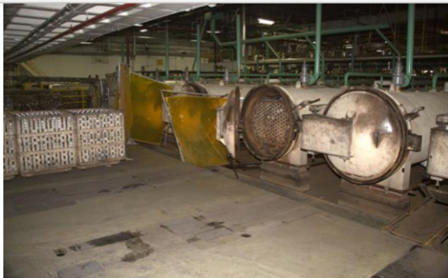
Exhibit 2. The large cylindrical steam pressure cooker called a retort.
